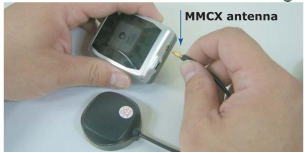
Under blocking area, the external antenna can extend the signal reception from HI-406BT-C
